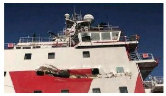
Damaged vessel (crew cabin) after allision with turbine foundation in German windfarm under construction.
