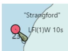
Safe Water physical AtoN including AIS. The presence of an AIS transmitted signal intended for use as an aid to navigation associated with a physical aid, including the AIS MMSI Number, can be obtained by cursor pick on the physical aid.
